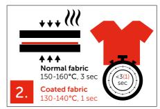
Pre-heat the fabric up to 3 or 1 seconds to remove residues, impurity and reduce shrinkage.
